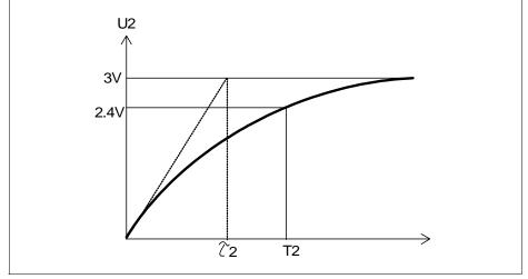
The voltage transient during the charging of  $C_2$  is shown in the following figure:
