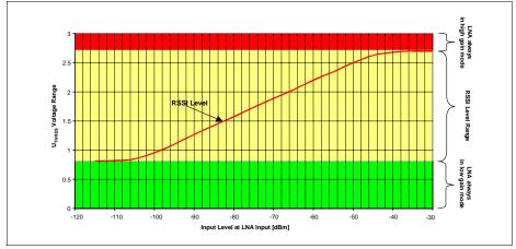
AGC and are used to charge an external capacitor which finally generates the LNA gain control voltage.
