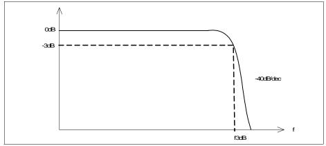
Figure 11 Frequency characteristic in case of ASK mode
