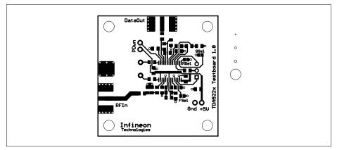
Figure 16 Top Side of the Evaluation Board
