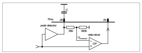
Figure 8 Data Slicer Threshold Generation Utilising the Peak Detector
