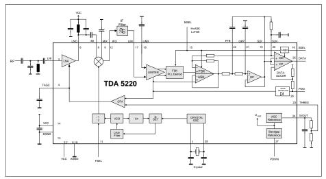
Figure 2 Block Diagram
