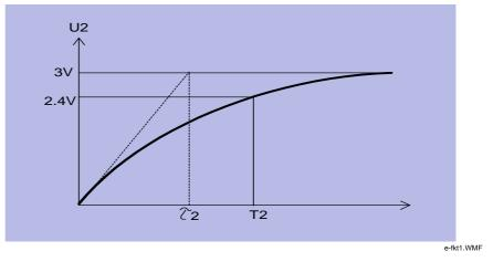
Figure 4-11 Voltage appearing on C2 during precharging process
