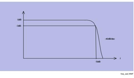
Figure 4-9 Frequency charcteristic in case of ASK mode
