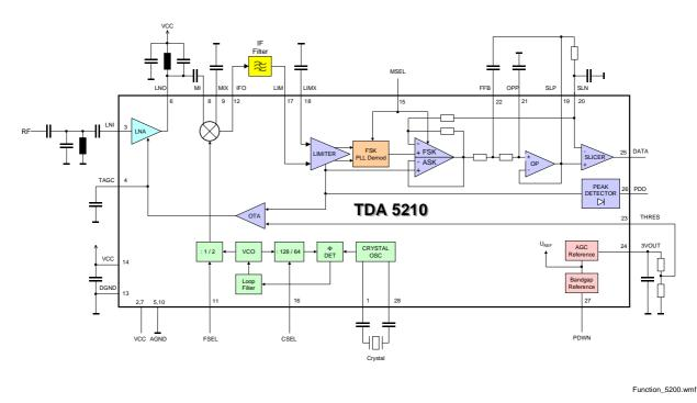
Figure 3-2 Main Block Diagram
