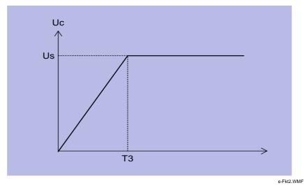
Figure 4-12 Voltage transient on capacitor C attached to pin 20
