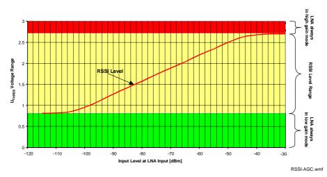
Figure 4-2 RSSI Level and Permissive AGC Threshold Levels
