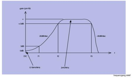
Figure 4-8 Frequency characterstic in case of FSK mode
