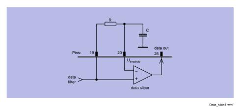
Figure 4-5 Data Slicer Threshold Generation with External R-C Integrator
