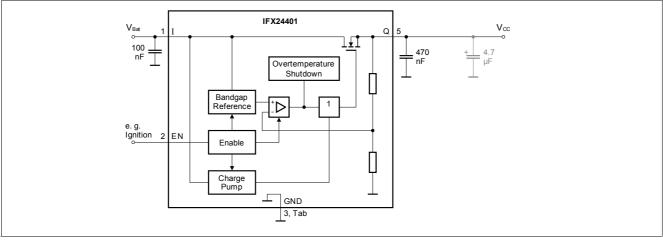
Figure 4 Application Diagram
