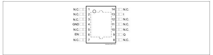
Figure 3 Pin Configuration PG-SSOP-14 (top view)
