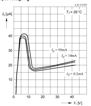
Current Consumption  $I_q$  versus Output Current  $I_Q$
