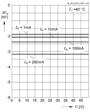
Line Regulation  $\Delta V_{\text{Q}}$  versus Input Voltage Change  $V_{\text{I}}$
