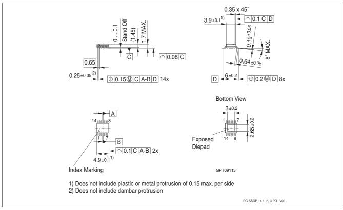
Figure 6 PG-SSOP-14
