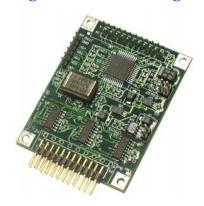
The 24/7 Data Acquisition Wildcard is your instrument's complete analog front end, offering exceptional resolution, excellent stability, and remarkable noise rejection. Ideal for high resolution, low frequency measurements, this I/O module accepts low level signals directly from transducers – it amplifies and conditions them – and it converts them with 24 bits of resolution with no missing codes performance.
