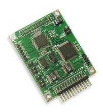
The **UART Wildcard** implements two full-duplex serial ports that can be configured for RS232, RS422, and RS485 protocols with data rates up to 56000 baud. Optional handshaking signals enable a modem connection for remote communications via any phone line. Dual 16-byte FIFO (first-in/first-out) buffers on each port reduce processor overhead when sending and receiving serial data streams.
