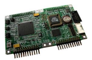
The PDQ<sup>TM</sup> Board is a fast I/O-rich computer that dramatically cuts the cost of data acquisition and control. It packs up to 1 megabyte of memory, communications, dozens of analog and digital I/O lines, and dual expansion I/O buses onto a compact low-cost board. This 2.5" x 4" single board computer is ideal for instrumentation, industrial control, automation, and data acquisition.
