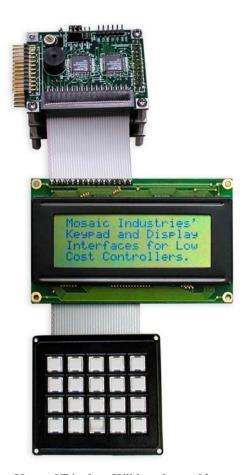
The **Keypad/Display Wildcard** provides a convenient interface to a 4 x 20 character display and 4 x 5 keypad.
