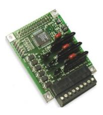
The **DC Solid State Relay Wildcard** gives you optically isolated control of up to three, 3-amp DC devices. Activation of solenoids, motors, pumps, heaters, relays, valves, thermoelectric coolers and fans is a snap with this Wildcard.
