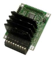
The AC Solid State Relay Wildcard gives you independent control of up to four, 5-amp AC devices.
