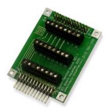
You can easily connect to the field side of any Wildcard using these handy screw terminals.
