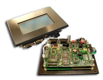
The QScreen<sup>TM</sup> Controller combines a C-programmable computer with a touchscreen-operated graphical user interface. Designed as a fully-functional industrial controller, the QScreen is ideal for OEM applications where installation space is critical, such as embedded systems, scientific instruments, robotics, and portable data acquisition. The QScreen can be commanded remotely from a PC or used stand-alone to provide real-time control of dozens of analog and digital I/O lines.
