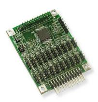
The **Digital I/O Wildcard** expands the digital I/O capabilities of Mosaic controllers. Up to 8 wildcards can be connected at once, increasing the number of I/O lines up to 160.
