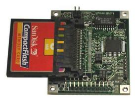
The Compact Flash Wildcard is ideal for applications that require large amounts of memory, the convenience of removable storage, and file-based data exchange with a PC. It allows you to plug in widely available Compact Flash memory cards that measure only 1.5" by 1.7" and hold many megabytes of nonvolatile data. Inexpensive form-factor adapters let you plug a CF Card into your laptop's PCMCIA socket for fast and easy file exchanges.
