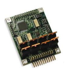
The heavy-duty **Power I/O Wildcard** provides eight high-current outputs and four high-voltage digital inputs. Inputs and outputs are optically isolated to  $\pm 2500$  volts. This versatile Wildcard makes it a snap to interface high voltage peripherals to your instrumentation or automation project.
