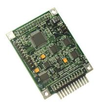
This general purpose **Analog I/O Wildcard** is ideal for controlling analog devices and actuators. It features eight channels unipolar, single-ended or four channels unipolar, differential 16-bit resolution analog voltage inputs and eight channels of 12-bit resolution analog voltage outputs. Inputs and outputs use onboard or external references, and the onboard references are optionally provided as excitations for external circuitry.
