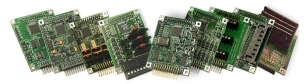
Mosaic's embedded controllers contain plenty of I/O for most applications, including serial ports, SPI, interfaces to graphics displays and keypads, analog I/O, and timer-controlled digital I/O lines.
